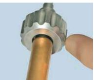
Ensure that the Fluted Nut (CES-SE-13 is assembled so that the Screw Extractor Compression Tube sits in the recess of the Fluted Nut.
