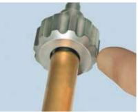
Ensure that the Fluted Nut is assembled so that the Screw Extractor Compression Tube sits in the recess of the Fluted Nut. 6 Attach the above assembly to the Straight or Offset "T" handle (CES-1-03/04).
