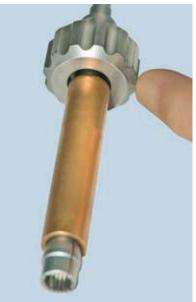
4 Followed by the Fluted Nut (CES-SE-13). Ensure that the Fluted Nut is assembled so that the Screw Extractor Compression Tube sits in the recess of the Fluted Nut.
