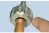
6 Followed by the Fluted Nut (CES-SE-13. Ensure that the Fluted Nut is assembled so that the Screw Extractor Compression Tube sits in the recess of the Fluted Nut.
