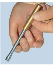
5 Select the corresponding Screw Extractor Shaft (CES-SE-01/14) and slide the Screw Extractor Compression Tube (CES-SE-12) over the Screw Extractor Shaft, followed by the Fluted Nut (CES-SE-13).
